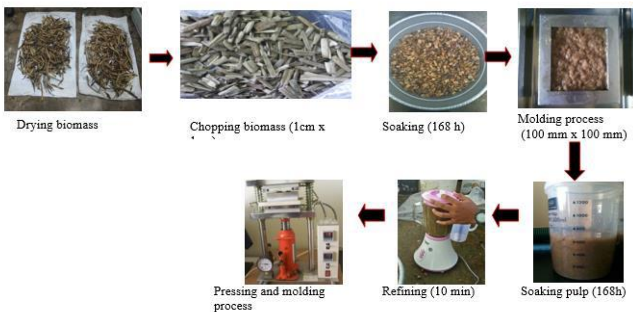
Fig 1: Biodegradabel board producing process
