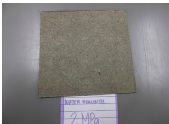
Fig 2. Water hyacinth bio-board successfully produce
