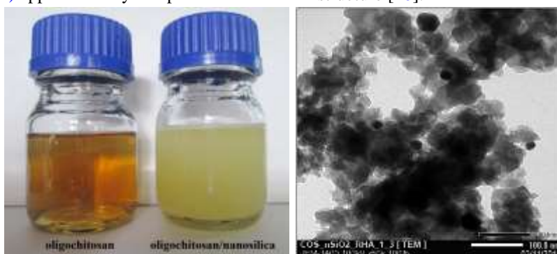
Fig.3: Photograph of 2% OC solution (left), mixture of 2% OC–2% nanosilica (right), and TEM image of OC–nanosilica.
