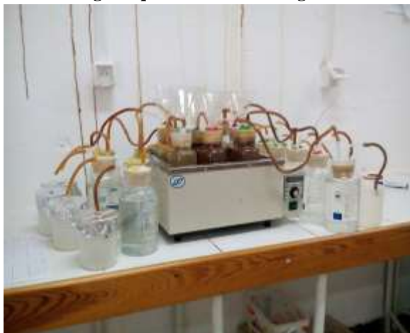
Fig.1: Experimental protocol for quantitative tracking of biogas produced
