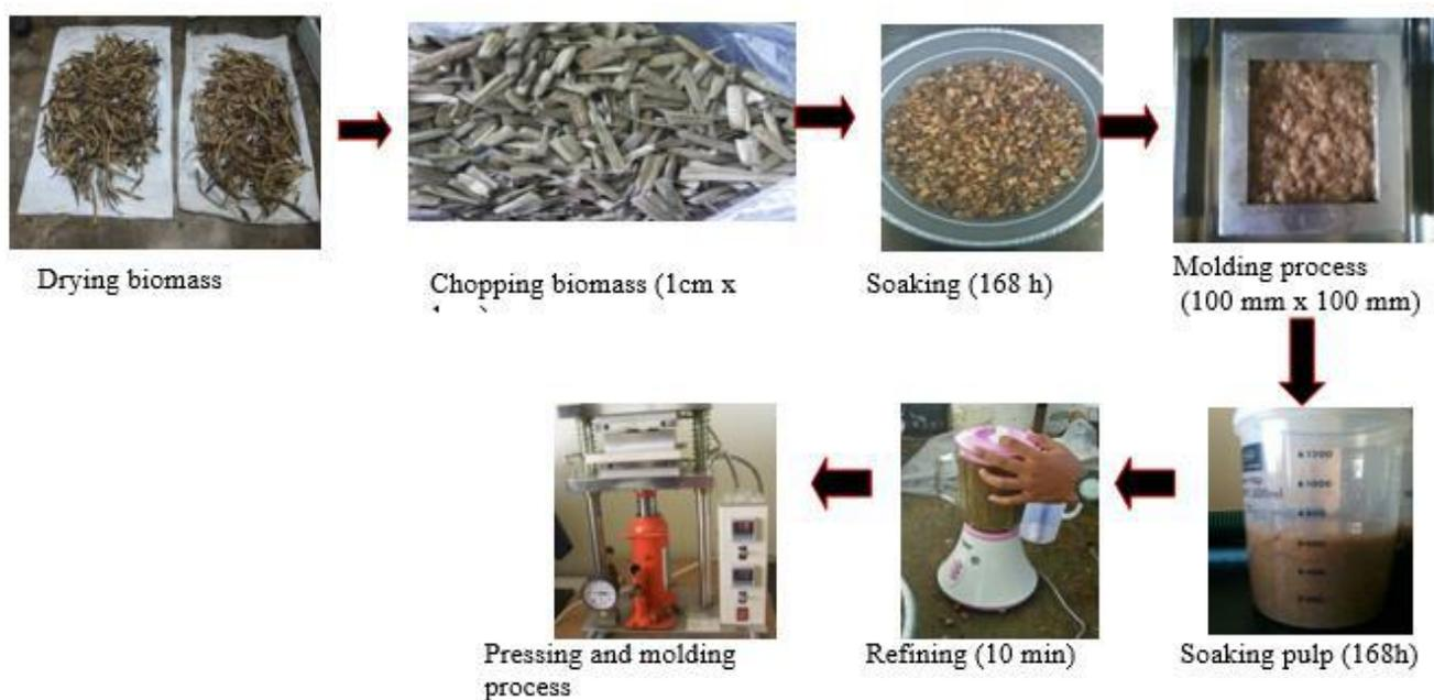
Fig 1: Biodegradabel board producing process
