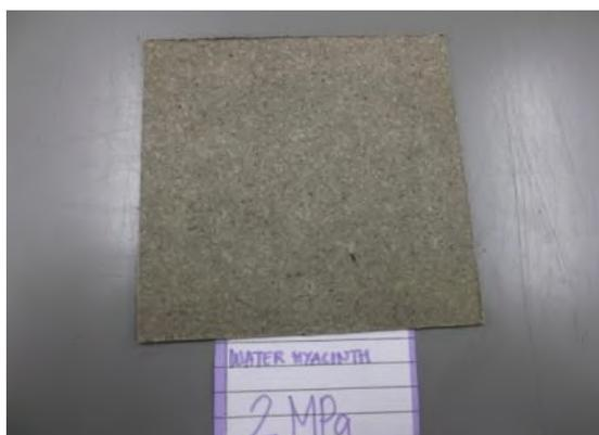
Fig 2. Water hyacinth bio-board successfully produce
