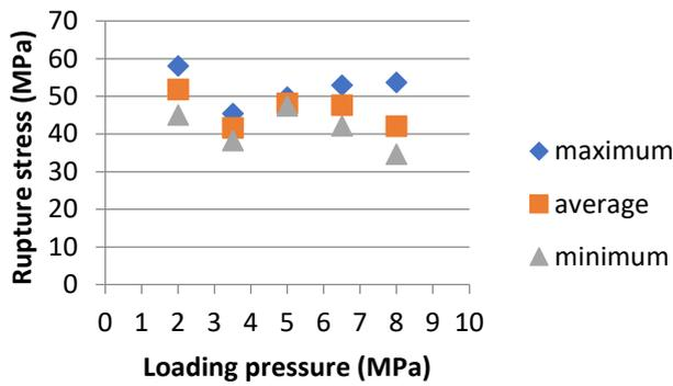
Fig 5. Water hyacinth bio-board rupture bending strength curve
