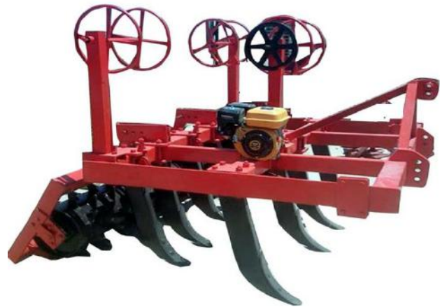
Fig.1: Combine implement used in instslation irrigation pipes
