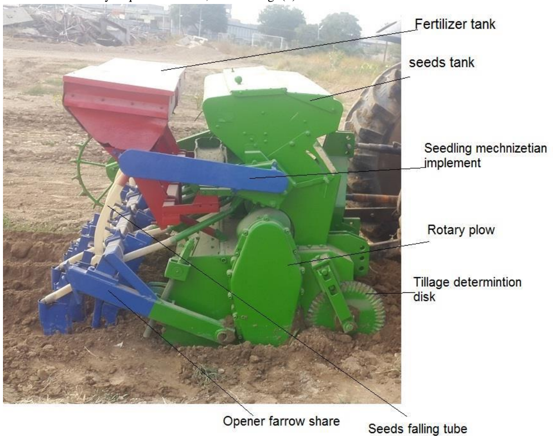
Fig.1: front view of the combine implement
