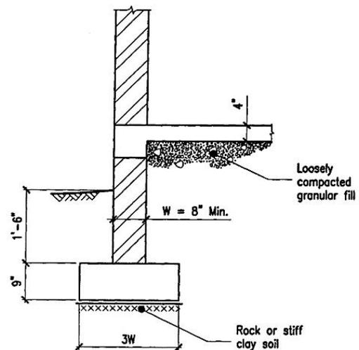
Fig. 5. Permissible arrangement of footing
