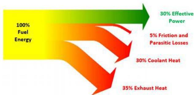
Fig. 16. Gasoline engine efficiency diagram ("Triple A" image)
