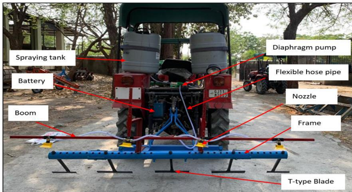
Fig.9 Developed sprayer cum weeder
