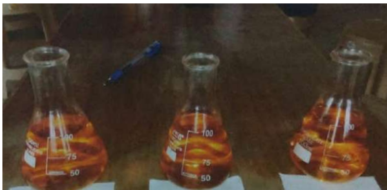
Fig 2.4 Petrol blends with different proportion of methanol
