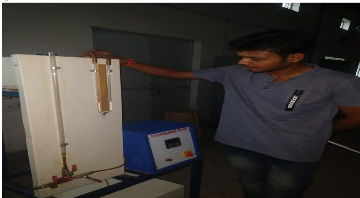
Fig .3.2 Fuel input measuring arrangement
