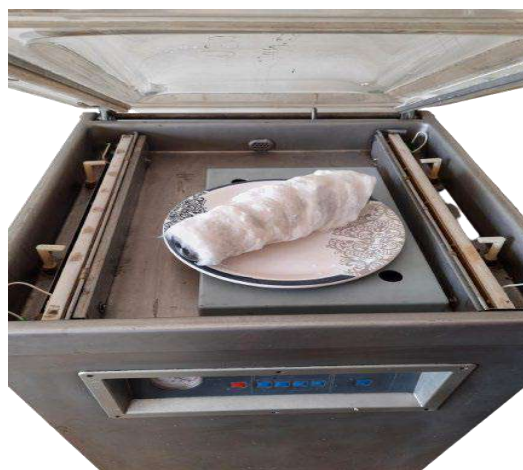
Fig. – 1 Cotton wrapped bottle inside vacuum machine
