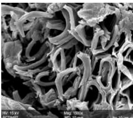
e. MW-assisted alkali pretreated leaf
