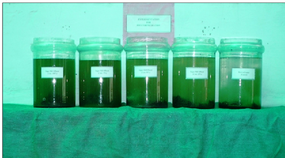
Plate 1: Phycoremediation treatment of sugar mill effluent using Spirogyra sp.
