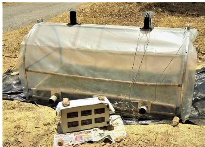
Fig. 4 Drying of mint leaves in LCSD
