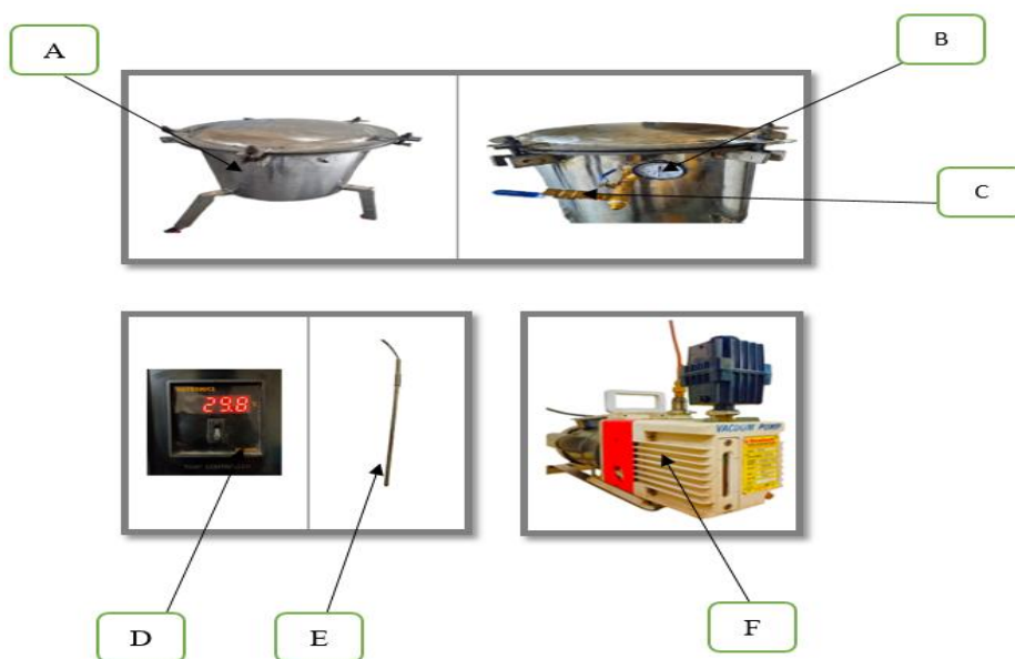
Fig. 2: - A - Vacuum chamber, B - Vacuum gauge, C - Valve, D - Display, E - Temperature sensor, F - Vacuum pump
