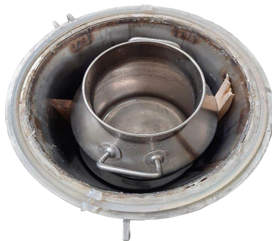
Fig. 3 The Can inside vacuum chamber
